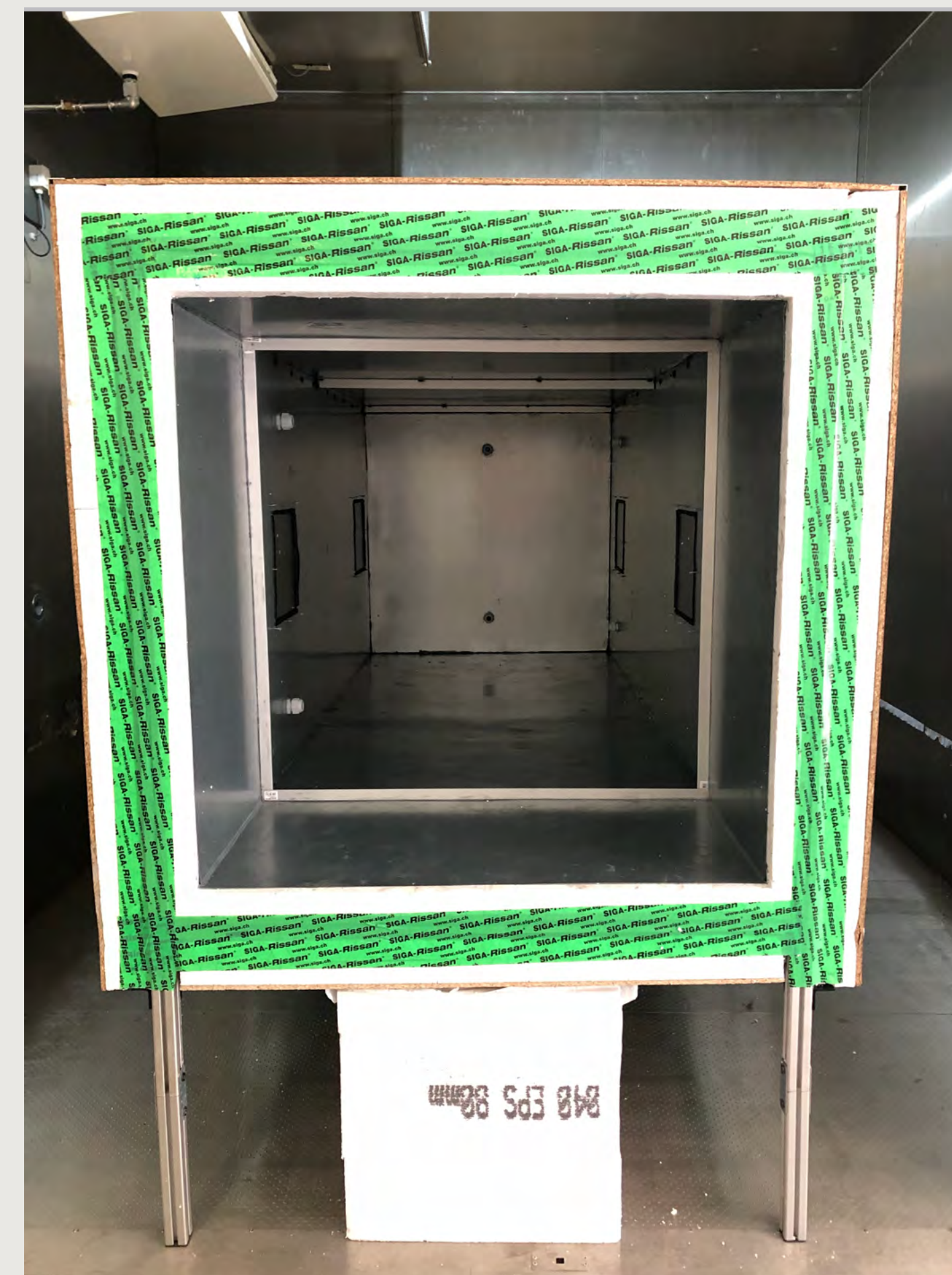
Built test box inside the climate chamber at
